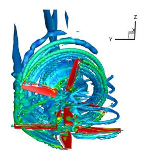
Fig. 1: Flow visualization around the rotor and propeller
