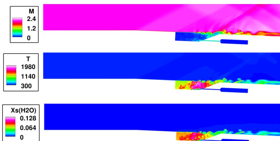
Fig. 1: Supersonic cavity combustion flow obtained by ILES. Instantaneous contours of Mach number (top panel), temperature (middle panel) and H 2 O mole fraction (bottom panel) are shown.
