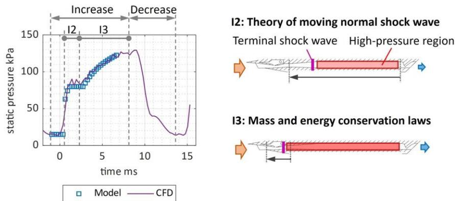
Fig. 1: Static pressure waveform of buzz upstream of exit nozzle, and schematic of pressure increasing period
