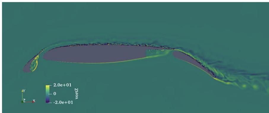
Fig. 2: Numerical analysis around 30P30N airfoil by RANS/WMLES hybrid method
