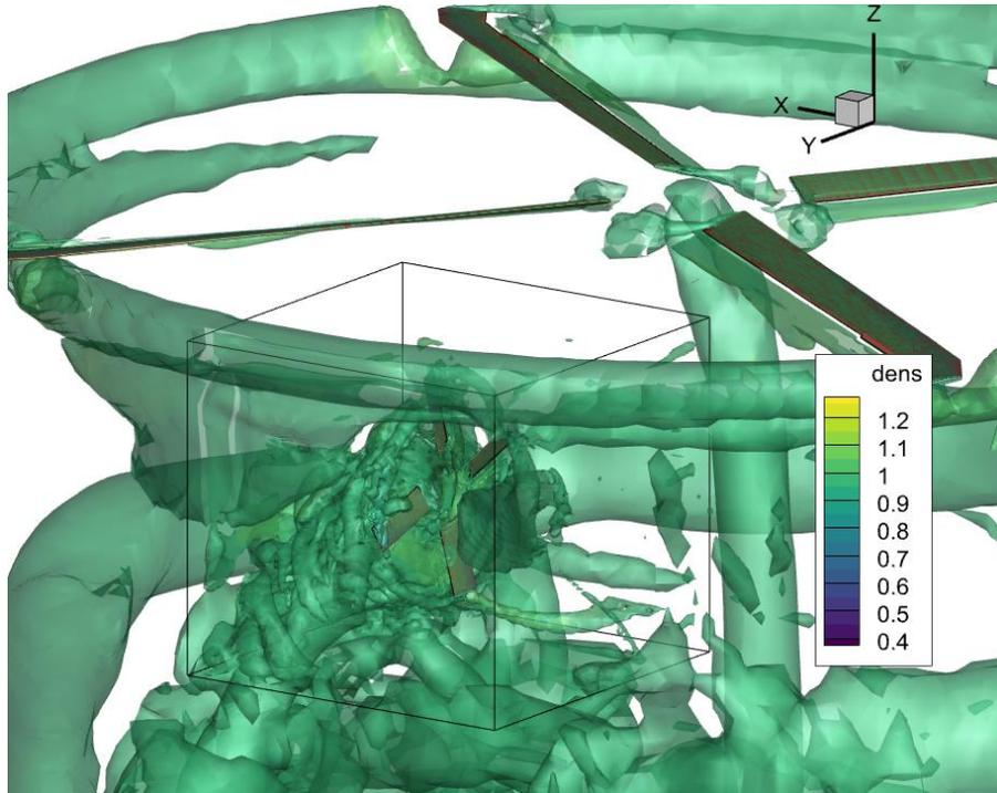
Fig. 1: Tip vortices visualization (Main rotor + side propeller, In hovering condition)
