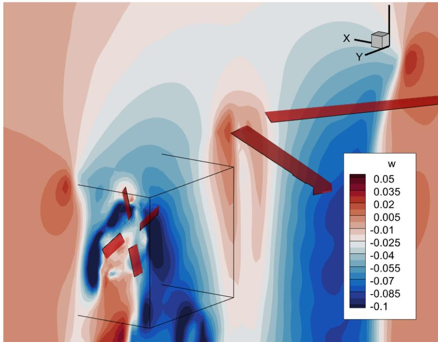
Fig. 2: Vertical velocity distribution (Main rotor + side propeller, In hovering condition)
