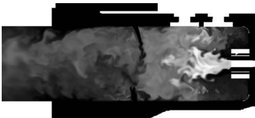
Fig. 2: Time-averaged temperature field of inner combustion chamber
