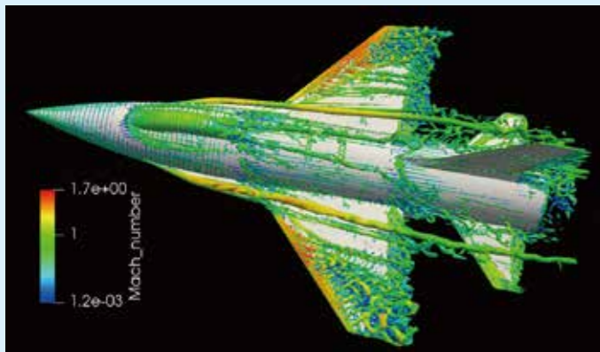
Iso-surface of Q criteria (color: Mach number)
