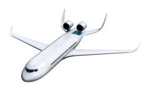
Fig. 1: JAXA Low-noise Technology-Reference-Aircraft 2035A (TRA2035A, 220-seat class) with a wide fuselage
