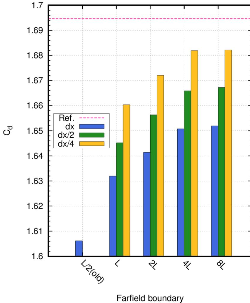
Fig. 1: Grid convergence of drag coefficient of prism (horizontal axis shows distant of outer boundary, color of the bar graph shows the minimum cell size, "Ref." shows the reference value obtained by using body fitted grid).
