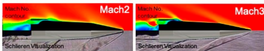
Fig. 2: Comparison between the CFD analysis results and the visualization results of the flow field in the wind tunnel experiment
