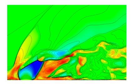
Fig. 2: Instantaneous static temperature contours.
