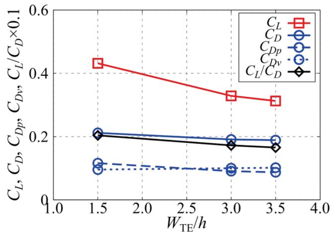
Fig. 3: Effect of  $W_{TE}/h$  on aerodynamic force coefficients.
