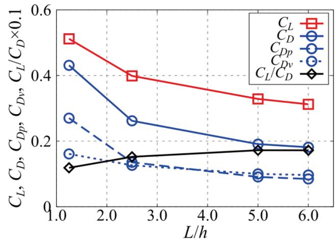
Fig. 4: Effect of L/h on aerodynamic force coefficients.
