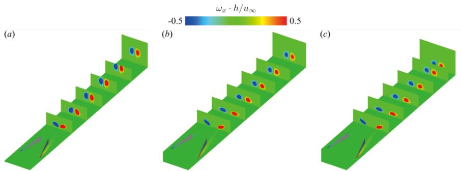
Fig. 2: Effect of  $L/h$  on distribution of streamwise vorticity: (a)  $W_{TE}/h = 1.5$ ; (b)  $W_{TE}/h = 3.0$  (baseline); (c)  $W_{TE}/h = 3.5$ . Cross-sectional contours are drawn every  $5.0h$  from trailing edge of VGs.
