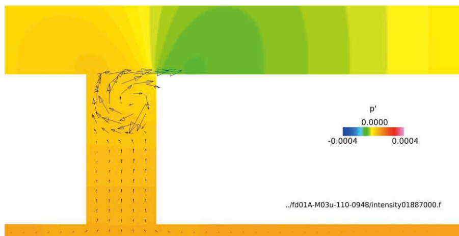
Fig. 1: The sound pressure and the velocity vector around the hole of the sound absorbing liner (Video. Video is available on the web.)
