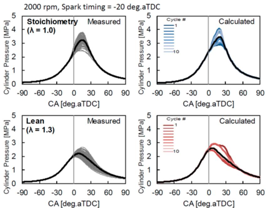
Fig. 2: Reproduction of pressure history (left) and cycle to cycle variation (right) of a mass-production engine for stoichiometric (upper) and lean (lower) conditions.
