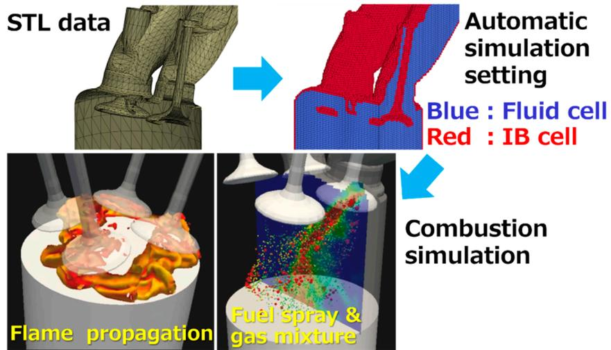
Fig. 1: Combustion simulation directly from engine data without meshing process.
