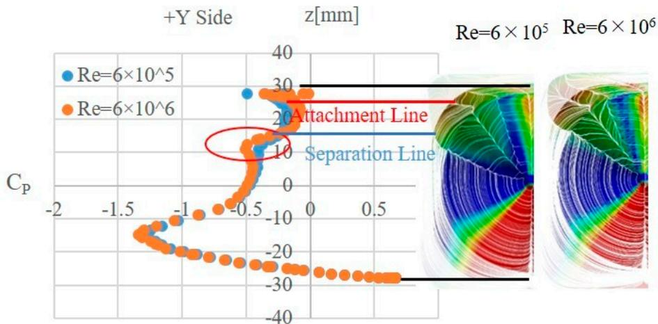
Fig. 2: Cut out of  $C_P$  (50AoA)
