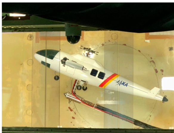
Fig. 1: Photo of the conceptual model during wind-tunnel testing
