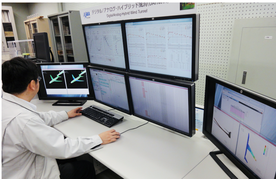
Fig. 1: EFD/CFD real time data monitoring using DAHWIN
