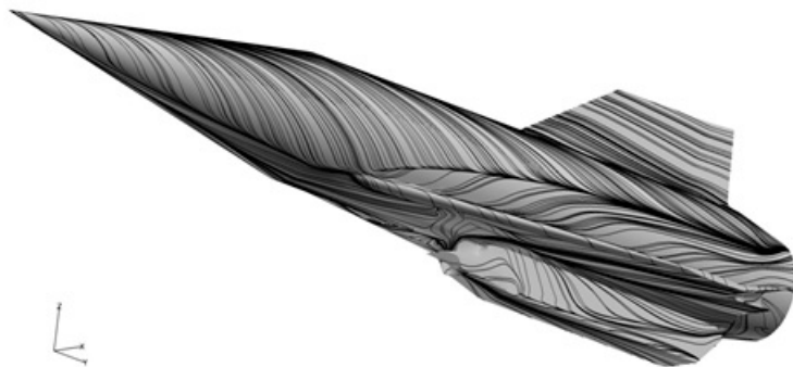
Fig. 3: High Mach Integrated Control Experiment (HIMICO) Vehicle with 15deg of elevator angle (HIMICO 2, Streamline, Mach5, AoA = -15deg)
