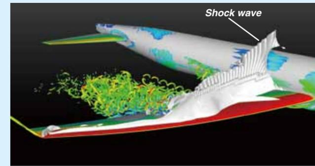
These simulation results visualize a flow around an aircraft flying at high angle of attack. The shock wave that appears above the wing during high-speed flight and the separated flow behind the shock wave are visualized. We found the shock wave oscillation (transonic buffet) and the fluctuation of separated flow behind the shock wave.
