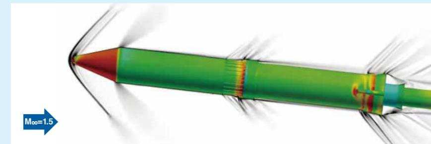
Flowfield (Attack angle: 5, Slip angle: 0, Roll angle: 0) computed  $C_p(-0.3 < C_p < 0.4)$  and density gradient magnitude
