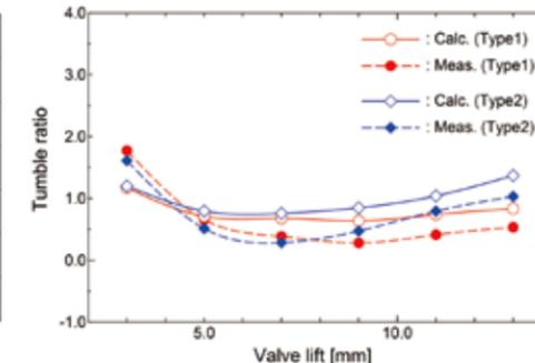
Effects of engine port shape difference reproduced by HINOCA. The type 2 is modified from type 1, aiming at augmentation of tumble flow even at the reduction of flow coefficient.
