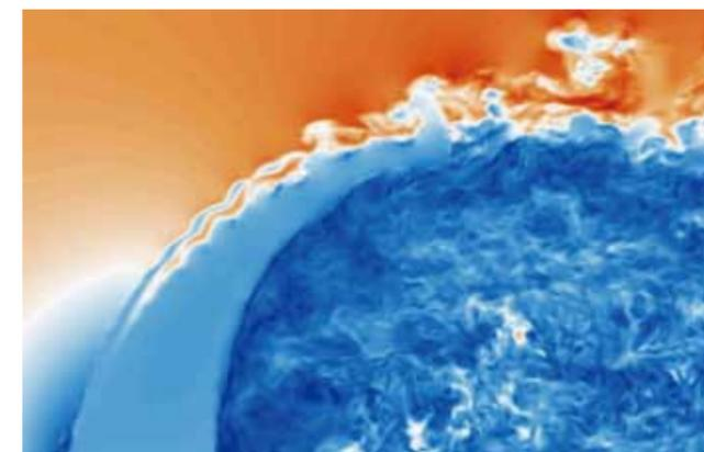
Visualization of liquid phase surface and velocity distribution near the fuel nozzle.
