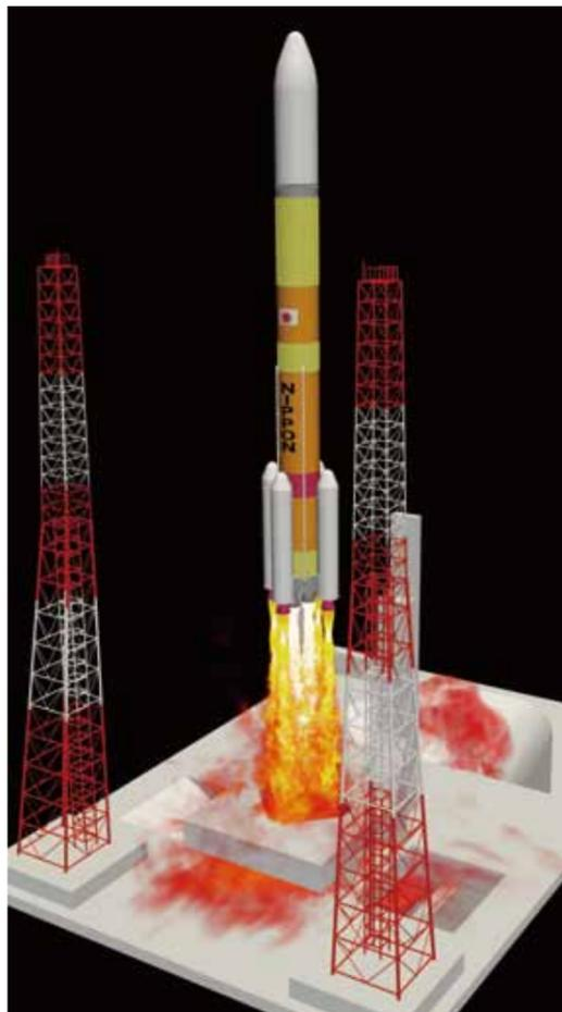
Computational fluid dynamics (CFD) is applied to analyze generation and propagation of acoustic wave generated from Japanese new flagship launch vehicle, H3, at lift-off. Exhaust jets of clustered liquid rocket engines and solid boosters are visualized by volume rendering of the temperature field. Acoustic field is shown by the pressure fluctuation, and it is found that the acoustic wave returns to the launch vehicle.
