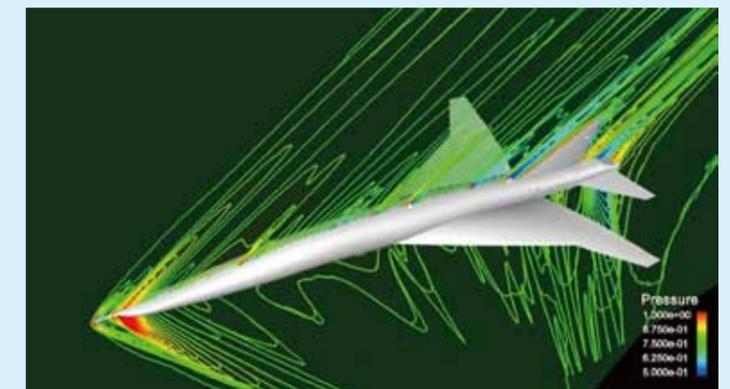
Shock waves from the D-SEND#2 airplane simulated for sonic-boom prediction
