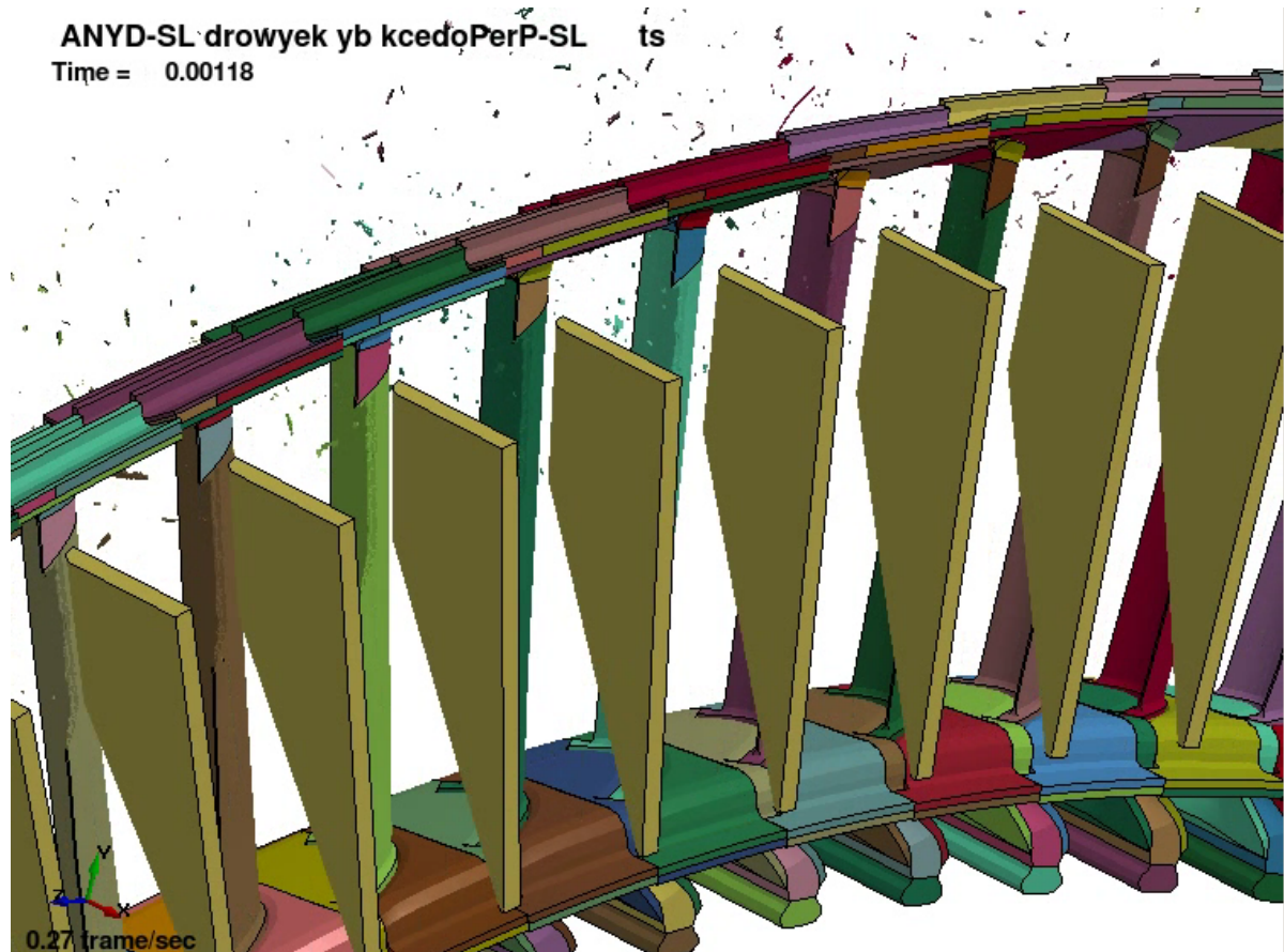
Fig.1 The fracture analysis of the cascade of CMC blades
