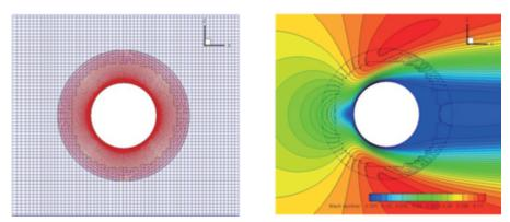
図1 Hole Cuttingと解析結果 : Hole Cutting and computational result
