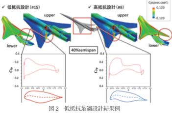
: Drag minimization design result. (Left: Low-drag geometry, Right: High-drag geometry)
