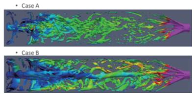
図2 乱流構造(Q値の等値面) : Structure of turbulence (Iso-surface of Q criteria)
