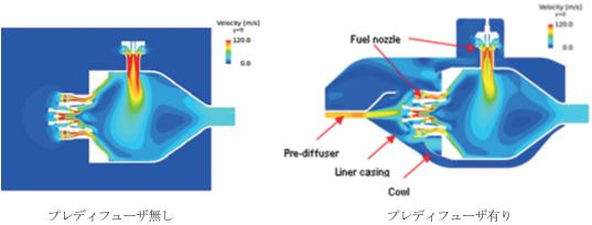
Without pre-diffuserWith pre-diffuser図1 プレディフューザの有無が燃焼器内部の速度場に与える影響: Effect of pre-diffuser to velocity field inside combustor
