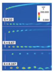
図 1 風車後流渦度分布 (上:周速比 $\lambda$ =10,中: $\lambda$ = 6.67,下: $\lambda$ =4.167) : distribution of wake vorticity (upper: $\lambda$ =10, middle: $\lambda$ =6.67, lower: $\lambda$ =4.167)
