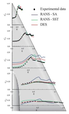
図1 デルタ翼上面の圧力係数分布 : Pressure coefficient distribution of a delta wing top surface
