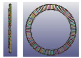
図1 全周動静翼干渉解析モデル : Analysis model (all turbine blades and stator vanes in one stage)
