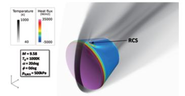
図1 カプセルRCSの数値計算結果 : CFD results of re-entry capsule with RCS
