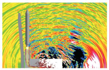
図1 イプシロン試験機1号機打上げ時の音響解析. (流体場:マッハ数,音響場:圧力変動) : CFD/CAA results for Epsilon launch vehicle at lift-off. (Hydrodynamic field: Mach number, Acoustic field: pressure fluctuation)
