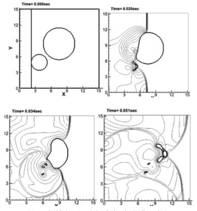
図2 二相流解析による水中の気泡の変形挙動の可視化 : Visualization of deformation of air bubbles in water by two-phase flow simulation.
