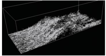
図2 剥離乱流 DNS の渦構造 : Vortical structures observed in DNS of a separated turbulent boundary layer.
