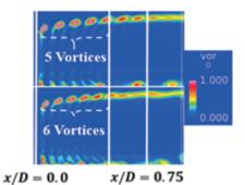
図1 渦度の分布(上図:2枚翼, 下図:3枚翼) : Vorticity distribution(Upper: Two-bladed rotor Lower: Three-bladed rotor)
