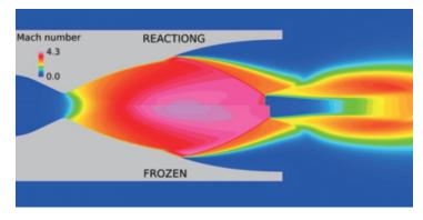
図1 ノズル圧力比45における等マッハ数線図,上段:反応流,下段:凍結流 : Mach number contours at NPR=45, Top: Reacting flow, Bottom: Frozen flow
